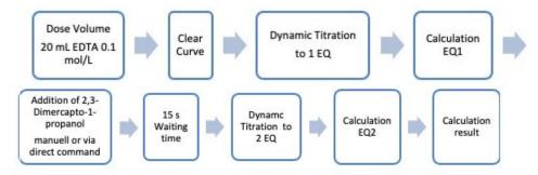
If the titration curve is too noisy at the beginning, a linear titration with 1 dosing step of 1 ml can be set as a pre-titration before the first dynamic titration.
