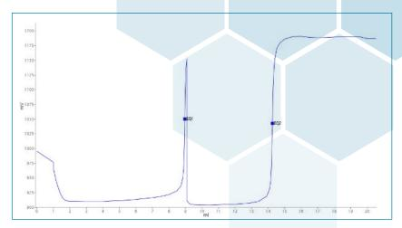
In Titrisoft, both equivalence points can be displayed in one titration curve. The following method sequence can be used for this:
